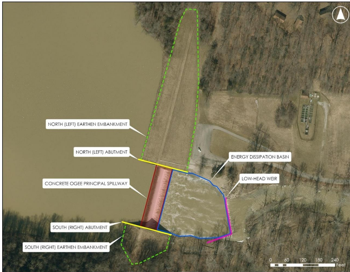
Figure 2. Versailles Dam Components
